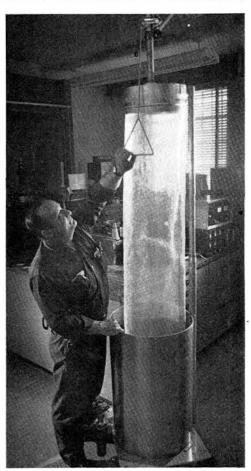
MAURICE (MO) ROBERT of General Maintenance Section 8222-2 resets valve of emergency shower after completing a test with Sandia-designed test fixture. One man can now conduct tests without risking water damage to surrounding research equipment.
